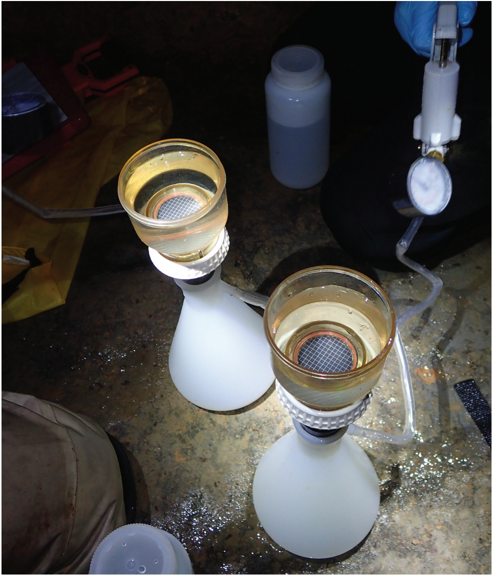
Figure 2. Filtration setup for eDNA collection. While wearing gloves, a 0.45- \mu m microbial filter was placed inside a filter funnel that was attached to a vacuum flask via a rubber stopper. A hand pump was used to create a vacuum and pull water through the filter. Filters were stored at room temperature in vials of 900 \mu l of Longmire's buffer (Longmire et al. 1997).
