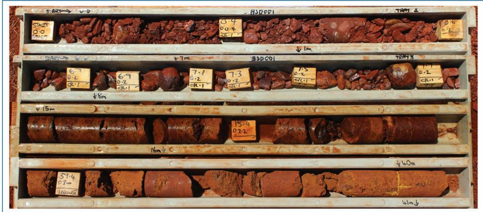
**Figure 1.** Diamond drilled geological core showing structure of the subterranean habitat from surface to 40 m depth.
